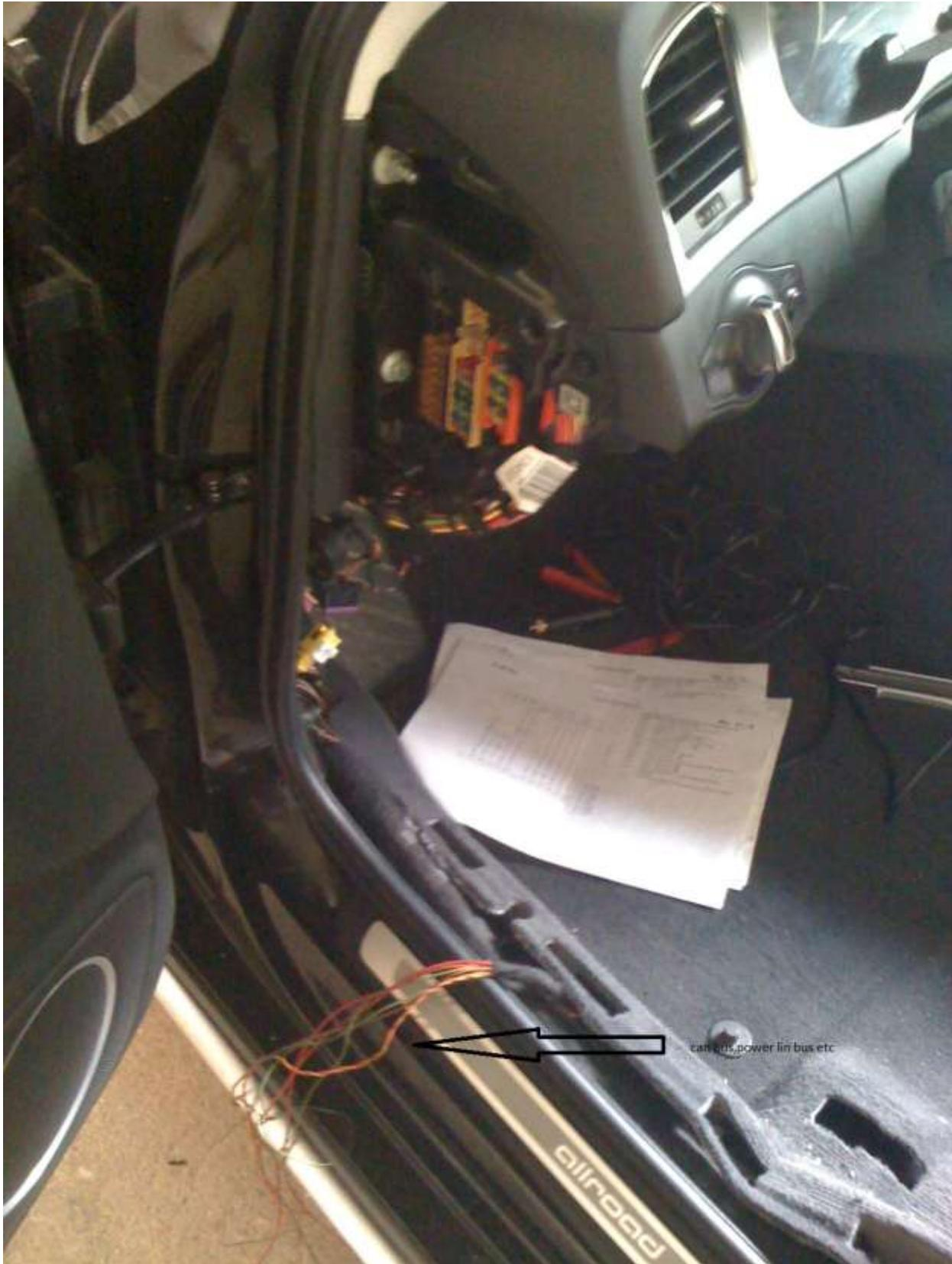
once i changed the side switch for the movement function i had to modify some wiring such as use only one red power cable to the memory controller input since there were more than 3 or 4 red power wires splitting from s44 into the non memory version function switch. I fold the others with tape so i do not cut any original version wires.(This way the modification is totally reversible)
