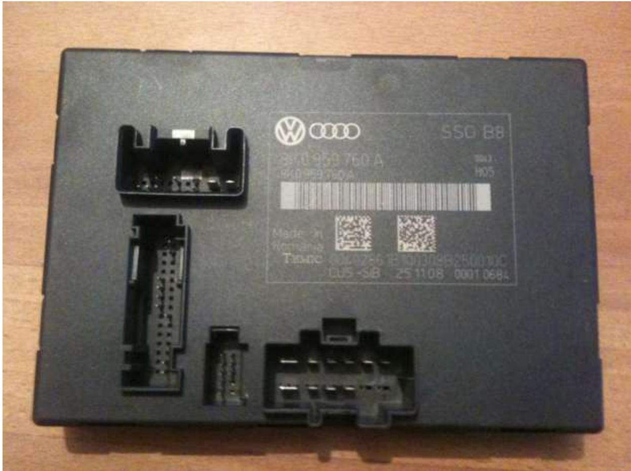
After i install the memory controller (using the same bracket that the j800 was in, i started connecting one by one all the corresponding wires. Please note that some basic electronic knowledge in schematic diagrams is required and you need to read and compare the 2 schematic diagrams of Elsa within the ventilation seat ,version page no 68 /1,5 and driver seat with memory function page 31/1,8 as well as the standard electric seat pin out configuration Elsa no 30/1 to 7.
